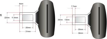
Length of metal tongue from end to where the metal starts to splay out.
